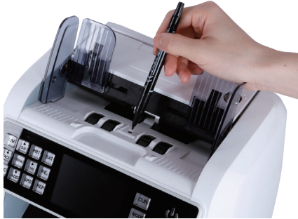
Figure 7 - 30 Use Marker Pen to Decrease the Sensitivity of Hopper Sensor
