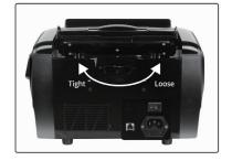
When banknote feeding is unsmooth or banknote counting is inaccurate, it can be solved through adjusting the vertical adjusting screw as well as the gap between resistance rubber and rubber wheel. Then you can put in a banknote and hold, if you feel the pull, the machine is workable.
